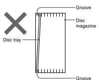
· Be sure all the trays are set in the magazine when using the unit.
